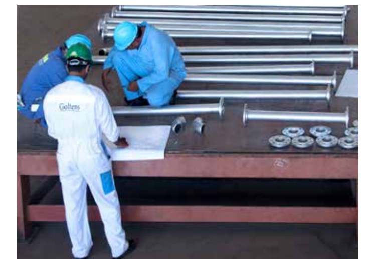
Goltens technicians performing quality checks on pre-fabricated piping prior to installation.
